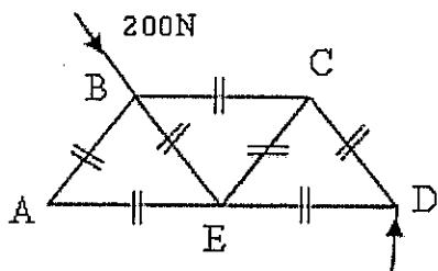
The framework ABCDE is smoothly hinged at A and is held with AD horizontal by a vertical force at D. A Force of 200N in the direction of BE is applied at B. Find the stresses in the rods BE ,EC and ED.
