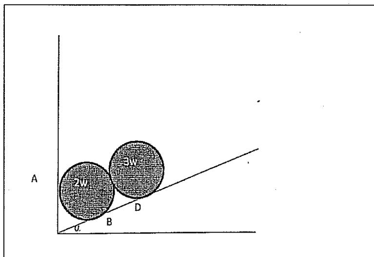
08. Two uniform cylinders of equal radius rest against each other on a fixed plane inclined at an angle  $\alpha$  to horizontal. The lower cylinder resting against a fixed vertical plane. The line of intersection of the planes is perpendicular to the section shown. The lower cylinder has weight  $2W$  and the upper cylinder has weight  $3W$ . Given that all the contacts are smooth, find the magnitudes of the reactions at all points of contact A,B,C and D.
