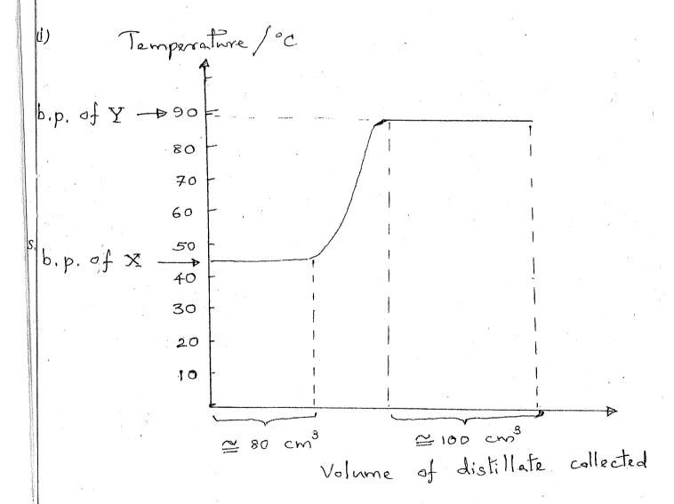
As you can see from this diagram, when a pure solvent is boiling, the temperature remains constant.
