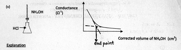
HCl is a strong acid which dissociates fully. Therefore the initial conductance is high due to  $H^+$ . When adding  $NH_4OH$ , the following reaction takes place.  $HCl + NH_4OH \longrightarrow NH_4Cl + H_2O$
