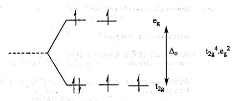
(ii) CFSE =  $-0.4 \times 4 \times \Delta_0 + 0.6 \times 2 \times \Delta_0$ =  $-0.4 \Delta_0 = -0.4 \times 200 \text{ kJ mol}^{-1}$ =  $-80 \text{ kJ mol}^{-1}$  (iii) Since compound is paramagnetic, it has unpaired electrons.
