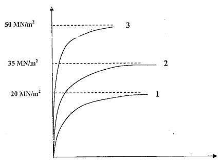
Curves 1, 2 and 3 correspond to normal loads of 5kg, 10kg and 15kg. The cross sectional area of the soil sample is  $0.002\text{m}^2$ .
