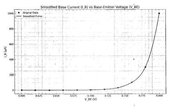
Estimate  $I_B$  when  $V_{BE}$  is 0.750 V
