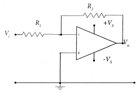
(i) Select the suitable resistance value for R<sub>1</sub> and R<sub>2</sub> from the values given below, So that the voltage gain of this OPAMP becomes 12.
