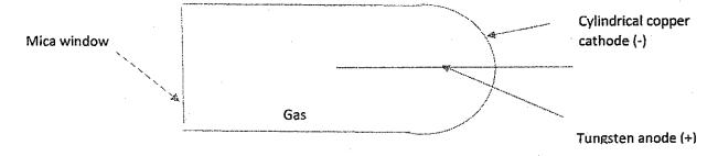
Radiation enters through the mica window, collides with gas atoms/moles, ionize them- primary electrons are produced which are accelerated towards the strong electrodes. The energetic electrons collide with other gas molecules creating further electrons (secondary), thus the cascade of ions and electrons create a pulse of current which can be counted.
