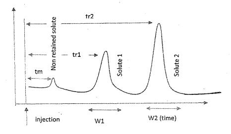
t<sub>m</sub> is the dead (or void) time; it is the time the void volume takes to pass through the
