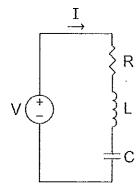
Net Impedance of the circuit is given by  $Z_{Net} = Z_R + Z_L + Z_C$
