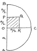
ABC is such a lamina with diameter AOB and OC is the radius perpendicular to AB. A square OPQR is cut out from the lamina, P being on OB and OP =a/2. R lies on OC. Find the centre of mass of the remaining part, the distance from OA and OC.
