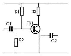
This circuit is activated with a dc power supply of 12 V. The base- emitter voltage of the transistor is 0.7 V and the base current;  $I_B=30~\mu A$ .
